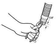
c. Open clamp. Twist hose back and forth while pushing down onto drain connector at the bottom of the washer. Continue until hose contacts the ribbed stop on the cabinet.
