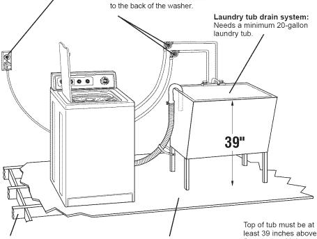
**Support:** Floor must be sturdy enough to support a total weight of 315 pounds (including washer, water, and load weight).
