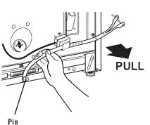
STEP 4. Cut the shipping strap about 16 inches from plug end. Look for the words "CUT HERE." Discard end with three cotter pins. Slide remainder of shipping strap from the electrical plug. You will use this to secure the drain hose.
