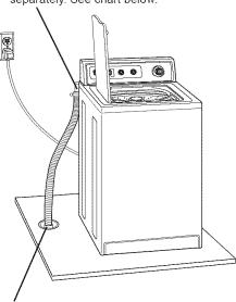
Floor drain system: Requires a siphon break, see chart below. A minimum carryaway capacity of 17 gallons per minute is required.
