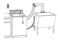
STEP 2. Locate the remaining piece of shipping strap (not the end with the three cotter pins) from STEP 4 of "REMOVE SHIPPING STRAP." Use it to wrap the drain hose together with the laundry tub or standpipe. Push fastener into the nearest hole in the shipping strap.
