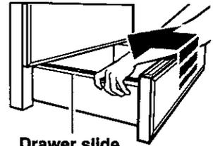
1. **Fit** ends of drawer slide rails into the drawer guides on both sides of opening.
