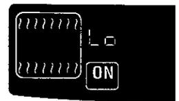
(example for Bake) ("Lo" is displayed after 5 seconds if oven temperature is below 170°F [77°C])
