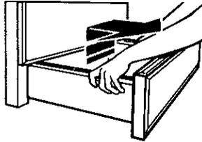
1. **Empty** drawer of any pots and pans before removing drawer. **Use** recessed area on top edge of drawer to pull drawer straight out to the first stop. **Lift** front and **pull out** to the second stop.
