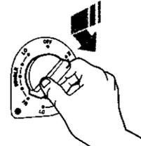
**To use the small element for smaller pans:** Push in and turn control knob to the left (counterclockwise) to the desired setting in the area marked "SINGLE".
