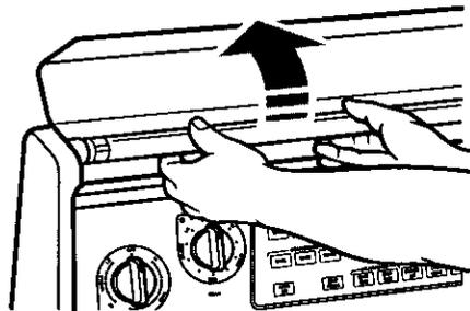
3. **Grasp** the fluorescent tube at both ends. **Turn** the tube approximately 90° in either direction until both ends come out of the receptacles. **Replace** with a 20-watt cool-white fluorescent tube.
