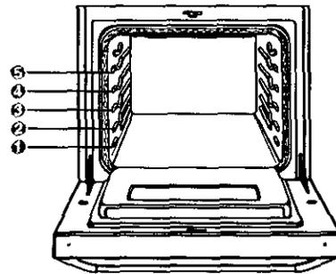
Your oven has three straight racks and five rack positions. Rack position 5 is the highest position, or farthest from the bottom of the oven. Rack position 1 is the lowest position, or closest to the bottom of the oven.
