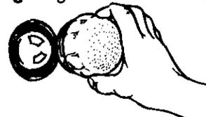
2. **Turn** glass bulb cover counter-clockwise to remove.
