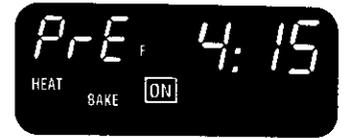
During the preheating time, the oven temperature rises to just about the temperature you set. As the countdown ends, the set temperature replaces "PrE" on the display. You will also hear a 1-second tone.
