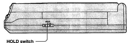
When this switch is slid toward the "HOLD" direction, the HOLD function (for preventing errors in operation) is activated. (If a function button is pressed when the HOLD function is ON, "HOLD" is displayed on the screen and the STANDBY indicator flashes.)
