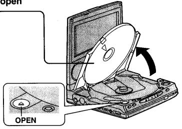
With the label side to be played facing upwards, (if the disc has a label) place the disc in position, using your fingers to push down on the area around the center hole.
