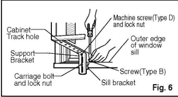
3. Using the M-screw and the lock nut, attach the support bracket to the cabinet track hole. Use the first track hole after the sill bracket on the outer edge of the window sill. Tighten the carriage bolt and the lock nut. Be sure the cabinet slants outward.
