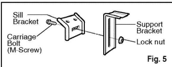
2. Attach the sill bracket to the window sill using the screws (Type B). Carefully place the cabinet on the window stool and align the center mark on the bottom front with the center line marked window stool.
