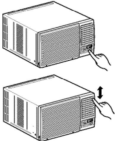
The direction of air can be controlled wherever you want to cool by adjusting the horizontal louver and the vertical louver.
