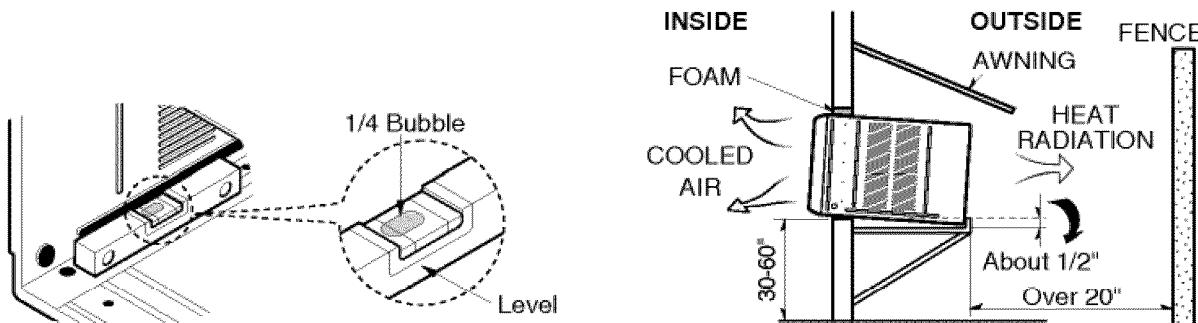
1. To avoid vibration and noise, make sure the unit is installed securely and firmly.
