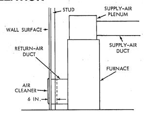
TYPICAL INSTALLATION USING DUCT EXTENSION
