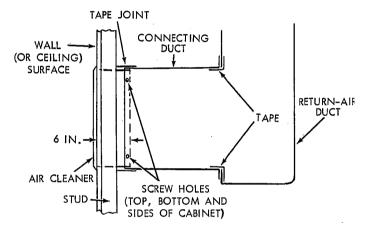
TYPICAL INSTALLATION USING DUCT EXTENSION
