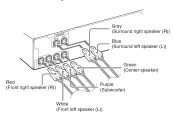
**2** Connect the speaker cord with the color tube to ⊕, and the speaker cord without the color tube to ⊝.
