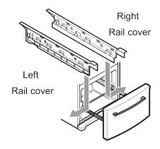
• Align the top holes of the rail cover with the top holes of the door supports to assemble the rail cover.
