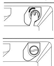
5. Turn the shutoff valve on (house valve).
