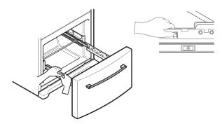
• Remove the screws(2) of the rail on both sides.
