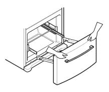
• With both hands, hold the center of the bar and push it in to let both rails fitted simultaneously.
