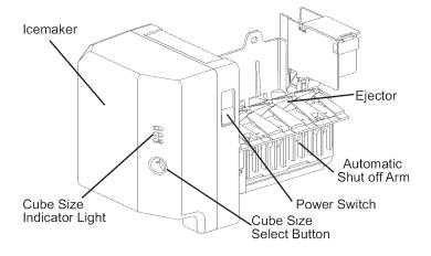
The icemaker will produce five cubes per cycle approximately 60-80 cubes in a 24-hour period, depending on freezer compartment temperature, room temperature, number of door openings and other operating conditions.
