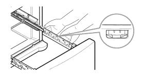
• With the drawer pulled out to full extension, insert the lower basket (4) in the rail assembly.
