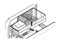
To Install, pull both rails out to full extension. Hook the basket supports into the rail tabs and push to the back of compartment.
