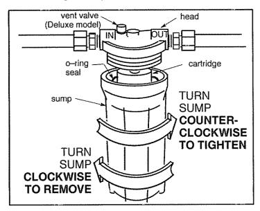
Note: A **special wrench** is available from Sears for removing the sump. See the parts list on page 9.
