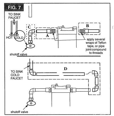
rag around assembly A to reduce heat transfer through the pipe, and into the head.
