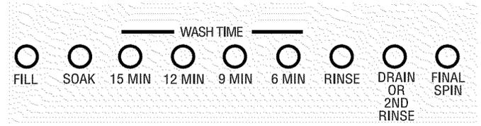
The Cycle Indicator Lights show what stage the washer is in. The wash time is the length of the wash agitation. The **6 MIN** light will remain lit during drain and spin. When the Selector knob is set to a new cycle the Indicator Lights will flash momentarily, showing what stages the cycle will go through.
