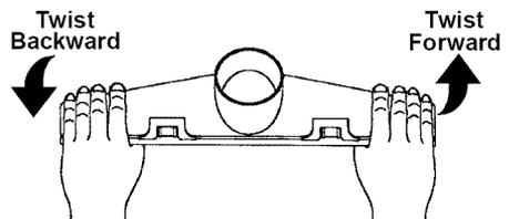
The wet nozzle assembly is ready for wet pickup use.
