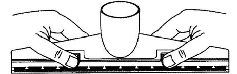
4. Inspect the pins of the insert to make sure they fit through the holes of the squeegee and fit into the matching slots in the nozzle body.
