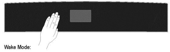
To wake the control, touch within the display panel. After 2 minutes without activity the control will beep and go back into sleep mode.
