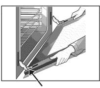
HINGE SLOT-Door removed from the appliance
