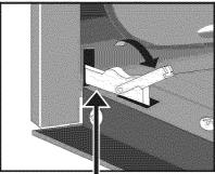
Lock engaged for door removal
