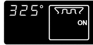
**NOTE:** Leave the door partly open whenever using the oven to broil. This allows the oven to maintain proper temperatures. If you want to change the broiling temperature after broiling has begun, repeat Steps 4, 5, and 6.
