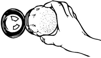
2. **Remove** the glass bulb cover in the back of the oven by screwing it out counter-clockwise.
