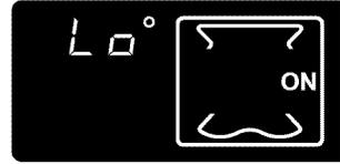
**NOTE:** After the temperature reaches 170°F, the red display will show the actual oven temperature at each 5°F increase and stop at the set temperature. To see the set temperature before it is reached, press the command pad you used to choose the cook setting. The set temperature will be displayed for 5 seconds.
