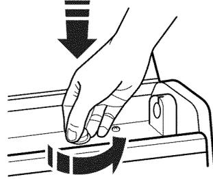
If the cooktop light still does not work, you may need to replace the starter. The starter is a knob-shaped part located on the right side of the backguard, under the light bulb. **To remove and replace the starter, first remove light bulb. Push** starter in and **turn** approximately 90° counterclockwise. **Pull** starter out of recessed area. You can find replacement starters at stores that sell fluorescent tubes.
