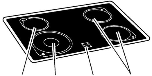
Standard elements    Dual element (some models)    Hot surface indicator lights    Halogen elements (Model KERH507 only)
