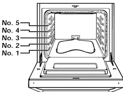
Your oven has two straight racks and five rack positions. Rack position 5 is the highest position, or farthest from the bottom of the oven. Rack position 1 is the lowest position, or closest to the bottom of the oven.
