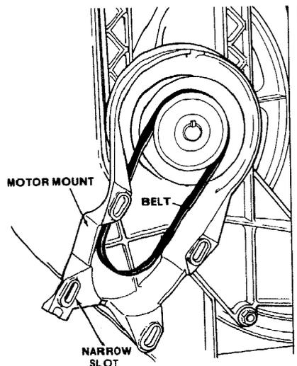
7. Carefully position the motor so that the poly "V" belt is around the motor pulley and the four motor studs align with the slots in the motor mount.
