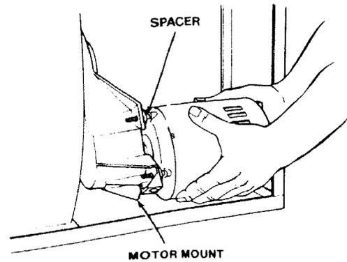
9. Install the threaded stud through the hole in the lower leg of the motor mount and over the motor stud as shown. Install the wing nut onto the threaded stud and turn wing nut until motor slides down tensioning the belt.
