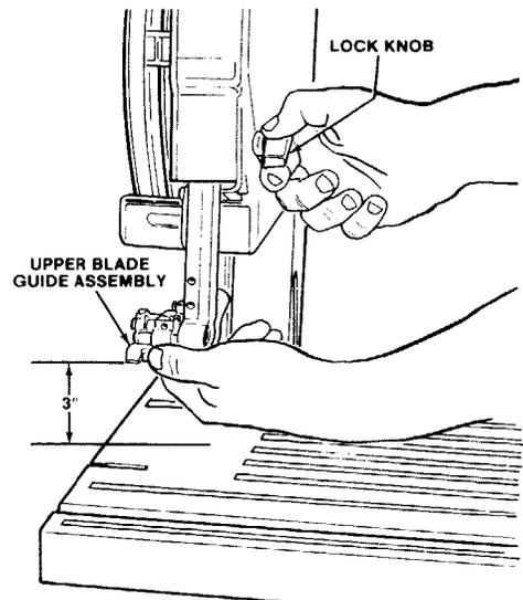
3. Loosen the two capscrews that lock the upper blade guides using a 1/8-inch hex "L" wrench and separate them about 1/8-inch. Repeat the same step for the lower blade guides.
