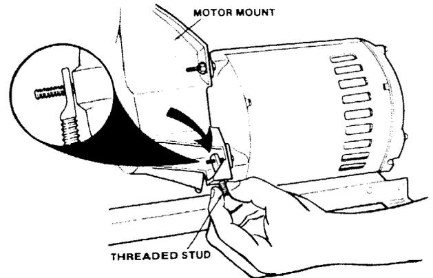
10. Install a flanged lock nut onto this motor stud. Tighten the flanged lock nuts, using a 3/8-inch wrench, until almost tight.
