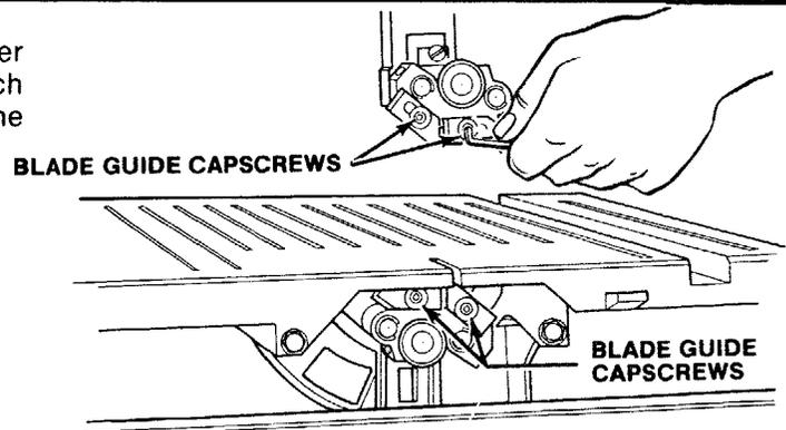
4. Loosen the setscrew which locks the blade guide support and push the support all the way back. Repeat for lower blade guide support.
