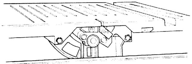
4. Slide the sanding platen into the blade slot in the table and fasten to the upper blade guide assembly where the right blade guide mounts. It may be necessary to loosen the left blade guide and slide it backwards until platen is in place.
