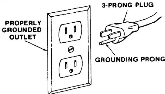
This power tool is equipped with a 3-conductor cord and ground type plug listed by Underwriters' Laboratories. The ground conductor has a green jacket and is attached to the tool housing at one end and to the ground prong in the attachment plug at the other end.
