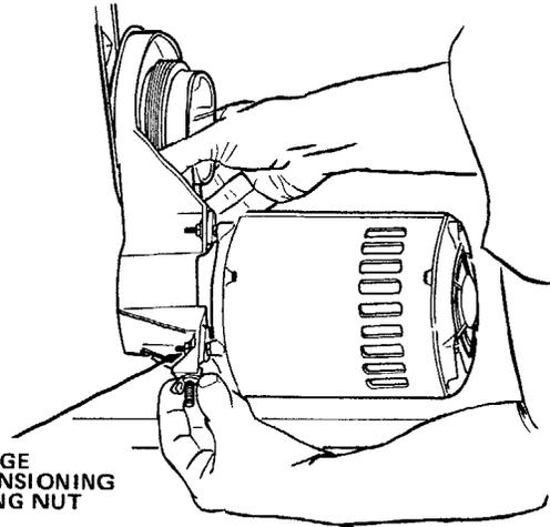
TIGHTEN FLANGE NUT AFTER TENSIONING BELT WITH WING NUT
