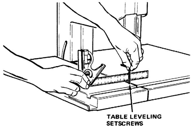
8. To keep the miter gage grooves in line, use a flat blade screwdriver against the head of one of the low head capscrews in the miter gage groove to force the table alignment key firmly forward into the notch in the front table.
