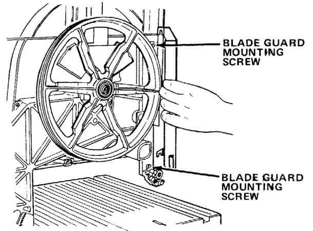
2. Loosen the upper blade guide assembly and lower to approximately 3 inches above rear table and retighten lock knob. This is necessary to make adjustments to blade guide and back up roller bearing.
