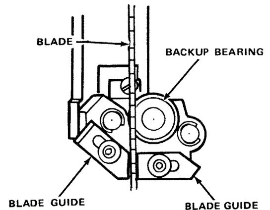
6. To insure the backup bearing is properly supporting the blade, push the bearing toward the blade until it almost touches it. Turn the upper wheel, by hand, checking the backup bearing to make sure it is not turning. If the bearing is turning the blade is too close. Move bearing slightly away from blade and tighten set screw with 1/8" hex "L" wrench. Turn upper wheel and recheck the bearing. Adjust again if necessary.
