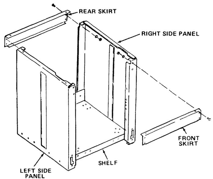
6. Secure rear of shelf to right side and left side panels using two (2) 1/4-20 x 1/2 truss head bolts, lockwashers, and hex nuts. Hand tighten nuts only at this time.
