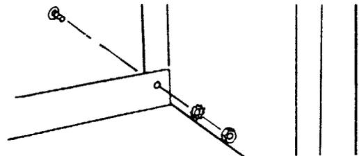
7. Locate the right and left side spacers, the six (6) 1/4-20 x 1/2 truss head bolts, lockwashers, and hex nuts. Position the spacer inside the right and left side panels and fasten in the three holes as illustrated. Tighten nuts with a 7/16" wrench or socket.
