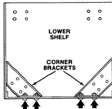
4. Locate the two (2) side panels, one (1) shelf stiffener, and six (6) 1/4-20 x 1/2 truss head bolts, lockwashers and hex nuts. Place the right side panel on its back side as illustrated. Stand up the lower shelf on the rear flange and line up the holes on the corner bracket and shelf stiffener with the holes in the side panel. Mount the bolts in the three holes and tighten hex nuts with a 7/16-inch wrench or socket. Repeat procedure for left side panel.
