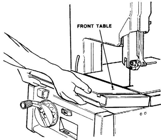
7. Use a 1/8-inch hex "L" wrench to adjust the two leveling setscrews to bring the rear edge of the front table up to the same height as the front edge of the rear table.
