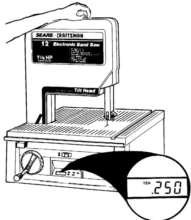
2. Turn the upper wheel by hand a few times and notice if the blade remains in the center of the tire on the top wheel.
