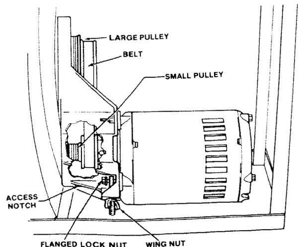
14. Belt tensioning is done by tightening the wing nut which pulls the motor down. The motor slides on the three (3) spacers and is locked in place by the flanged lock nut at the threaded stud.
