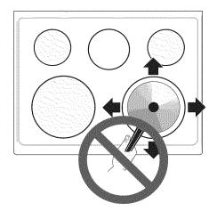
Sliding aluminum or copper clad bottom pans on the cooktop can cause metal markings on the cooktop surface. These marks should be removed **immediately** after the cooktop has cooled using the cooktop cleaning cream. Metal marks can become permanent if not removed prior to future use.
