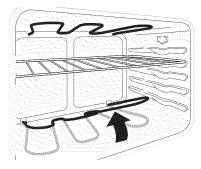
(For some models) If the lower bake element is visible it may be tilted up about 4 or 5 inches to clean the oven bottom.
