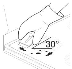
If soils remain, carefully scrape soils with a metal razor blade scraper, holding scraper at a 30 degree angle to the surface. Remove loosened soils with cooktop cleaning cream and buff surface clean.
