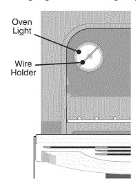
The oven light automatically turns ON when the door is opened. The oven light may also be manually operated by pressing the oven light switch located on top of the control panel. The oven light bulb is located at the rear of the oven and is covered with a glass shield held by a wire holder. The glass shield must be in place whenever the oven is in use.
