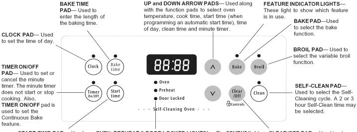
START TIME PAD— Used to set the desired start time for baking & Self-Clean. May be used with BAKE TIME to program a delayed bake cycle.
