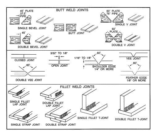
Figure 3. Types of Weld Joints
