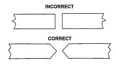
Figure 2. Workpiece Preparation
