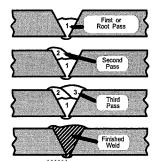
Figure 13. Triple Pass V Butt Joint
