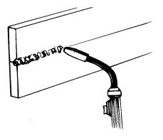
Figure 10. Horizontal Position Weld
