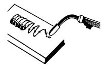
Figure 8. Weave Weld Bead
