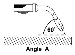
Figure 4. Gun Position, Angle A
