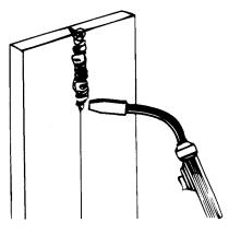
Figure 11. Vertical Position Weld
