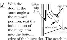
edge of the hinge slot. The notch in the hinge arm must be fully seated into the bottom of the slot.
