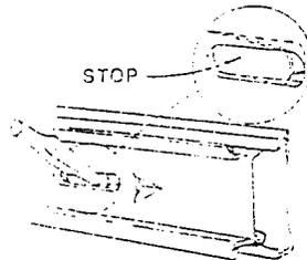
A. Pull drawer all the way open. B. Insert screwdriver behind the spring stop, twist out and down to hold the stop out on both slides and remove drawer. To reinstall drawer, reverse procedure.
