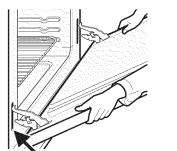
HINGE SLOT - Door removed from the oven Figure 2
