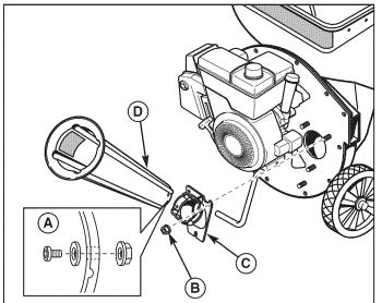
Figure 18. Installing the Chipper Cone
