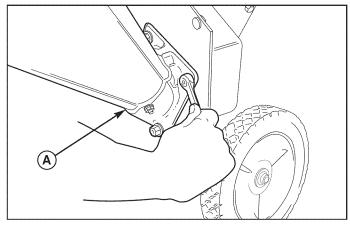
Figure 8. Inspect Chipper Knives A. Chipper Cone
