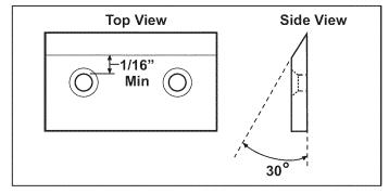
Figure 17. Chipper Knife Minimum Cutting Edge
