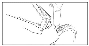
Figure 15. Installing the Chipper Cone
