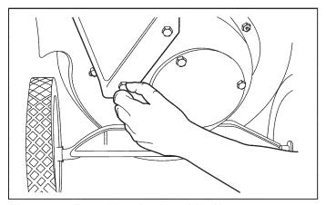
Figure 12. Removing the Shredder Hopper
