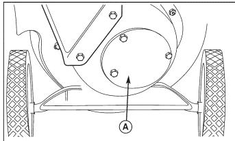
Figure 5. Inspect Shredder Hammers A. Access Panel
