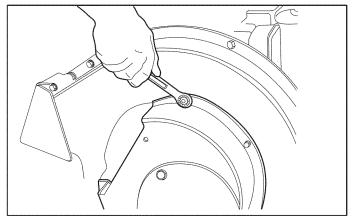
Figure 13. Removing the Rotor Housing
