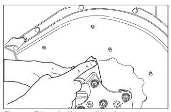
Figure 6. Triangular Hammer Wear Area
