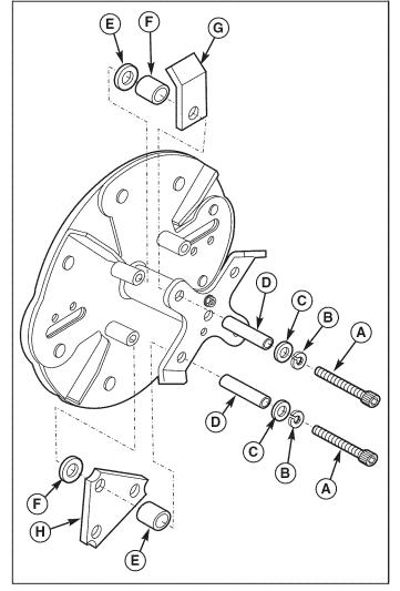
Figure 14. Removing the Rotor Housing
