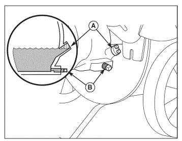
Figure 11. Oil Fill and Oil Drain
