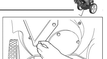
Figure 19. Attaching the Hopper
