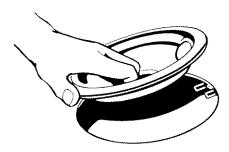
3. Hold the coil element as level as possible with the terminal just started into the receptacle. Push the coil element terminal into the receptacle.
