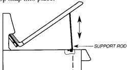
**To lower cooktop:** Hold the front edge of the cooktop and carefully push back on each support rod to release. Then gently lower the top into place. The support rods will slide into the range frame.
