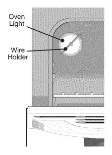
The oven light automatically turns ON when the door is opened. The oven light may also be manually operated by pressing the  $\binom{\text{Oven}}{\text{light}}$  pad.
