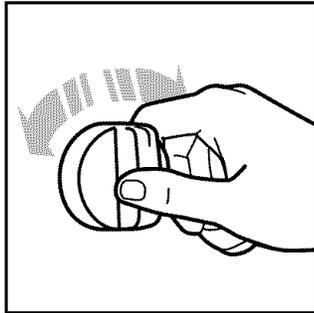
**NOTE:** The ACCUSIMMER™ control knob does not have to be pushed in before turning.
