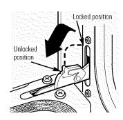
Pull the hinge locks down to the unlocked position.
