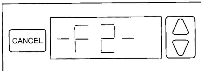
A fault code indicates that there may be a functional error. As a safety precaution, the control will automatically cancel the program. Follow the procedures described below to check the range.
