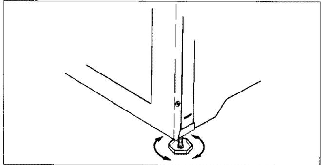
**WARNING:** To reduce the risk of accidental tipping of the range, it must be secured by a properly installed anti-tip device. To check if the device is installed properly, use a flashlight and look underneath the range to see that one of the rear leveling legs is engaged in the bracket slot. The anti-tip device secures the rear leveling leg to the floor, if properly engaged.
