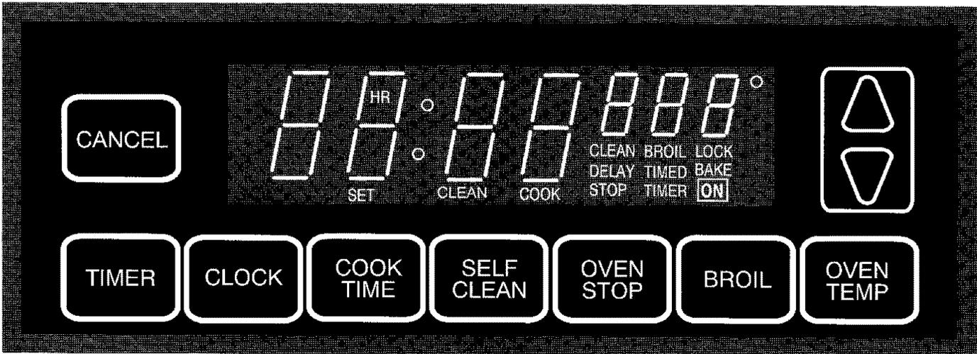
The electronic clock and oven control on your Maytag range is used for the time-of-day clock, timer, bake, broil, delay start and self-clean functions. A beep will sound each time a function pad is pressed. At the end of an operation, consecutive beeps will sound.
