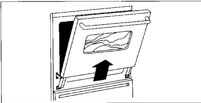
**CAUTION:** Hinge arms are spring mounted and will slam shut against the range if accidentally hit. **Never place your hand or fingers between the hinges and the front oven frame.** You could be injured if the hinge snaps back.
