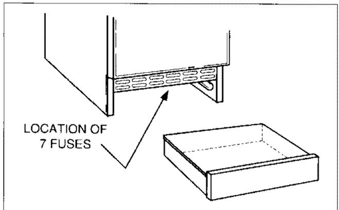
If part of your range does not operate, check to see if a fuse has blown. A gap in the fuse strip or a darkened window indicates a blown fuse. Replace with the same type and amperage "P" fuse.
