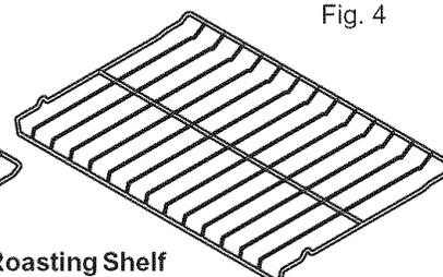
Place **Roasting Shelf** with care (some models; See Fig. 2). Be sure the Roasting Shelf is level and the front end of the shelf rests over the front ends of the oven rack glides on both sides of the oven interior (See Figs. 3 & 4).
