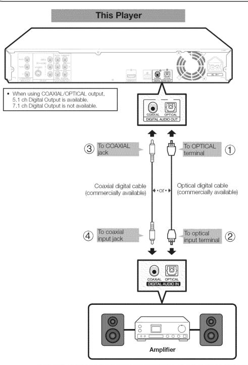
Audio equipment with a digital audio input terminal or jack
