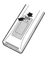
2 Load the two R-03 size batteries ("AAA" size, UM/SUM-4) supplied with the remote control unit. Make sure that the battery poles ⊕ and ⊖ are positioned as indicated.
