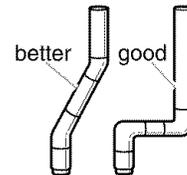
4. Use clamps to seal all joints. Do not use duct tape, screws or other fastening devices that extend into the interior of the vent to secure vent.
