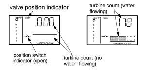
TURBINE OPERATION: If no water is flowing through the softener, the turbine indicator displays three zeros. When water is flowing, the flow bar scrolls across the display, and a 000 to 140 count repeats for each gallon of water passing through the turbine. To check for positive operation of the turbine if zeros are shown, open a nearby **soft** water faucet and observe the turbine count and flow bar.
