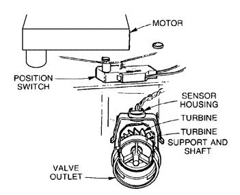
POSITION SWITCH STATUS: With the valve in service, or any of the recharge cycles, the switch indicator will show open →. While the valve is rotating from 1 position to another, the indicator will show the switch closed →. A defect is probable if indications vary from this pattern.
