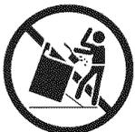
**⚠ WARNING** Stepping, leaning or sitting on the doors or drawers of this range can result in serious injuries and also cause damage to the range. Do not allow children to climb or play around the range. The weight of a child on an open door may cause the range to tip, resulting in serious burns or other injury.
