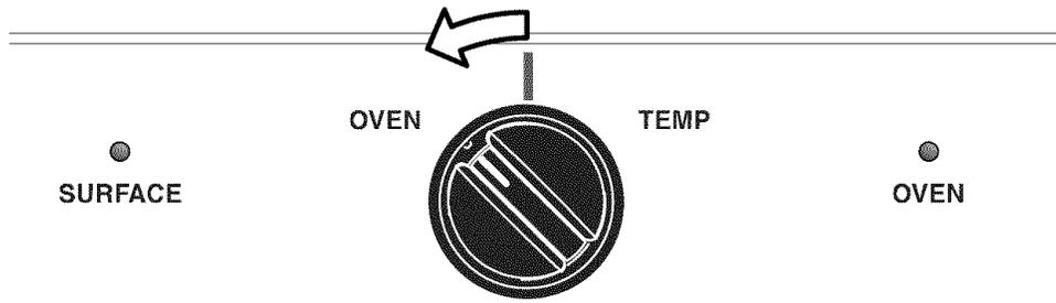
**READ THE INSTRUCTIONS CAREFULLY BEFORE USING THE OVEN.** For satisfactory use of your oven, become familiar with the various functions of the oven as described below. Note: The **Oven** indicator light will glow when the oven is turned on when baking or broiling. A quick glance at this indicator light when cooking is finished is an easy check to be sure the oven is turned off.
