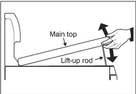
**CAUTION** When lowering the lift-up range top, grasp the sides with finger-tips only. Be careful not to pinch fingers. **DO NOT** drop or bend the range top when raising or lowering. This could damage the surface.
