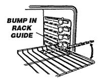
placed correctly in the oven, the guides have a bump to prevent the racks from tilting. Your oven has four (4) rack positions that may be used during cooking.
