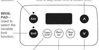
TIMER ON/OFF PAD-Used to set or cancel the PAD-Used minute timer. The minute timer does not start or stop cooking.
