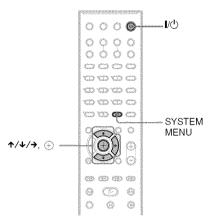
After connecting the AC power cord (mains lead), the demonstration appears in the front panel display. When you press I/O on the remote, the demonstration turns off.
