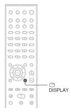
Use the Control Menu display to select a function and to view related information. Press 🖱 DISPLAY repeatedly to turn on or change the Control Menu display as follows:
