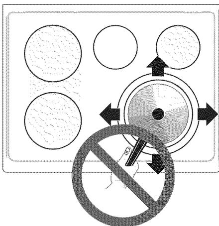
Sliding aluminum or copper clad bottom pans on the cooktop can cause metal markings on the cooktop surface. These marks should be removed **immediately** after the cooktop has cooled using the cooktop cleaning cream. Metal marks can become permanent if not removed prior to future use.
