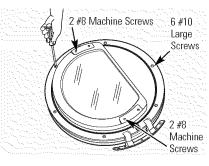
**5.** Remove the 6 large tapping screws (#10) located around the perimeter of the door outlining the gasket, and the 2 machine screws (#8) on the hinge side.
