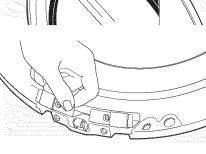
**15.** Place the hinge cover in position. Align the hinge cover holes with the holes in the door.
