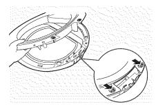
**7.** Unlock the 4 tabs on the plastic cover and separate the plastic cover from the frame.
