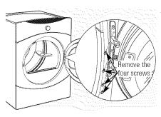
**2.** Open the door to approximately 90 degrees. Remove the 4 screws starting from the bottom to the top. Make sure the door is supported while removing the screws.
