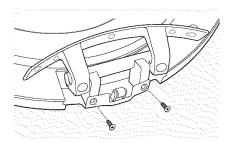
12. Loosely fasten the hinge assembly to the edge using 2 machine screws (#8).
