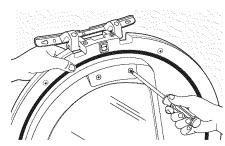
**13.** Hold the door on its side with one hand and fasten the remaining 2 screws as shown. Then tighten the 2 screws (#8) holding the hinge assembly.
