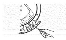
**10.** Remove the hinge assembly by removing the 2 machine screws (#8) that fasten it to the frame. Pull the hinge assembly out and set it aside.
