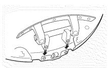
**11.** Place the hinge assembly in the opposite side of the door. Align the hinge holes with the door holes.
