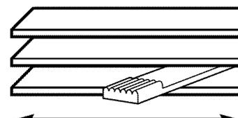
To open the vent, push the lever to the right.
