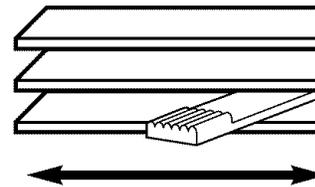
To open the vent, push the lever to the right.
