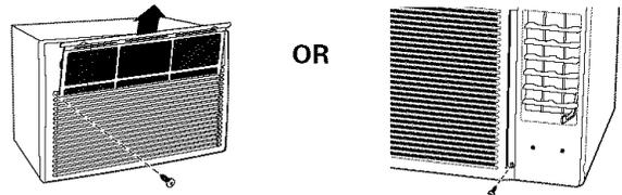
On models with a raise-up inlet grille, lift it (see the Care and Cleaning section) and remove the screw behind it (if present) that holds the grille in place.
