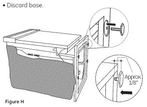
• Screw leveling legs back into the dishwasher frame, approximately 1/8" from frame as shown.
