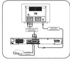
NOTE: When in AUX1 or AUX2 mode, only composite video sources will have video output signal, therefore, connect only RCA video output or TV Out to your TV sets
