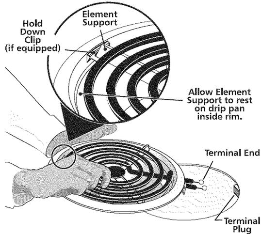
**CAUTION** Be sure the range is cool before removing elements or drip bowls. Be careful not to bend terminal ends when replacing elements after cleaning.
