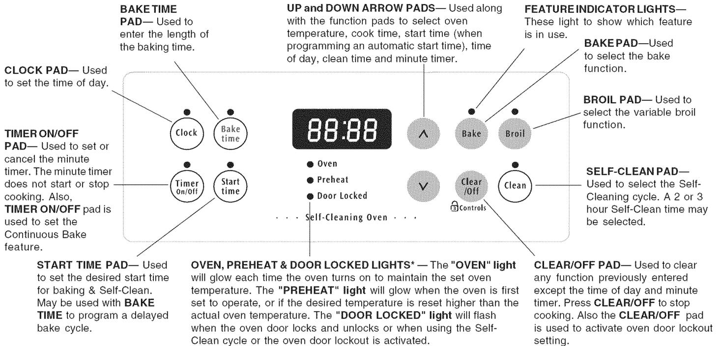
\*Note: The **OVEN** indicator light on the electronic display will turn ON & OFF when using the Bake feature & during preheat. This is normal & indicates that the oven is cycling to maintain the selected baking temperature. When the preheat indicator light turns OFF, your oven is ready.
