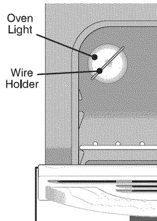
**CAUTION** Be sure the range is unplugged and all parts are COOL before replacing oven light. Wear a leather-faced glove for protection against possible broken glass.
