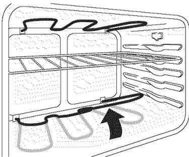
The baking element may be tilted about 4 or 5 inches to clean the oven bottom.
