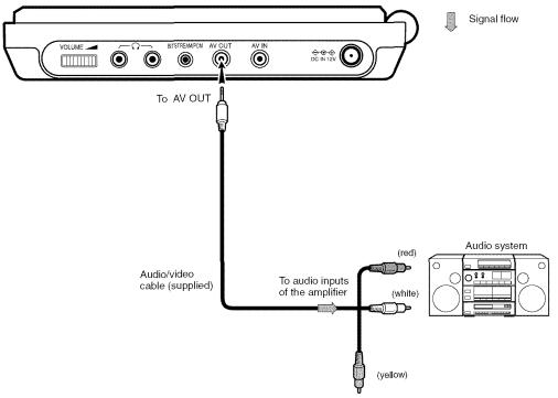
When the AV OUT or BITSTREAM/PCM jacks are connected to the audio input terminals of an audio system, sounds of discs can be heard on the connected audio system. For instructions on connections to audio systems, see [57).
