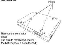
4 Turn the battery pack over and insert four catches into the player's corresponding holes ①. Then, slide the battery pack in the direction of the arrow ② until a "click" is heard.
