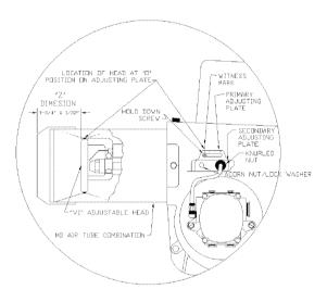
BECKETT AFG BURNER ELECTRODE ADJUSTMENTS F-HEADS
