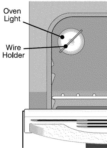
For models equipped with the interior oven light, the light bulb is located at the rear of the oven and is covered with a glass shield held by a wire holder. The glass shield must be in place whenever the oven is in use.
