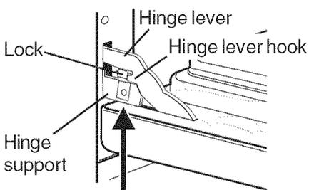
Lock engaged for door removal
