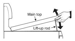
range top, grasp the sides with finger-tips only. Be careful not to pinch fingers. **DO NOT** drop or bend the range top when raising or lowering. This could damage the surface.
