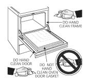
Use soap & water to thoroughly clean the top, sides and front of the oven door. Rinse well. You may use a glass cleaner on the outside glass of the oven door. **DO NOT** immerse the door in water. **DO NOT** spray or allow water or the glass cleaner to enter the door vents. DO NOT use oven cleaners, cleaning powders or any harsh abrasive cleaning materials on the outside of the oven door.
