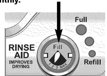
the cycle is adjustable by moving the lever inside the reservoir area. For most water conditions use the manufacturer recommended setting of "2". Adjust it up to the "MAX" setting for hard water. Set the lever anywhere between these amounts as needed to get the best results. Replace the cap and turn it clockwise to close.
