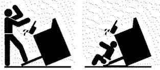
If your range is removed for cleaning, servicing or any reason, be sure the anti-tip device is re-engaged properly
