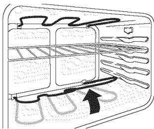
Baking element may be tilted about 4 or 5 inches to clean oven bottom.
