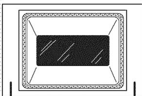
*Do not rub or clean the door gasket—it has an extremely low resistance to abrasion.*
