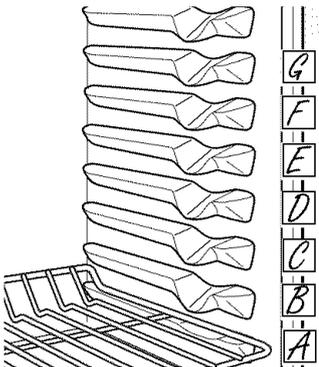
**To remove a rack,** pull it toward you, tilt the front end up and pull it out.
