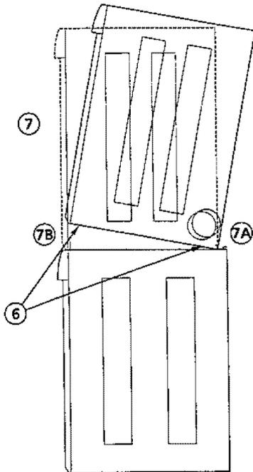
8. Insert the 2 long screws provided in the kit through the holes in the dryer front panel and install into the front mounting brackets.
